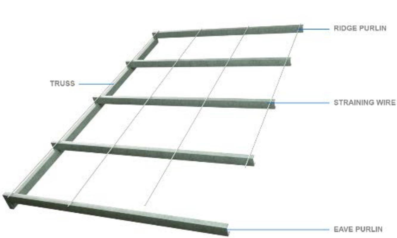
**Fix PVC coated straining wire from the top apex purlin, over intermediate purlins to the bottom eave purlin at 383 mm centers. First straining wire to be fixed 50 mm away from gable end. Evenly tension all wire ensuring that cut ends face downwards.**
