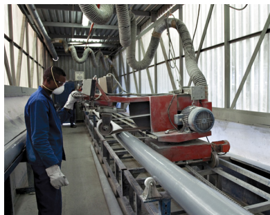
Machining of cured pole
