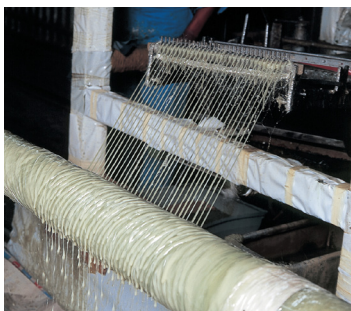
Winding of glass filament
